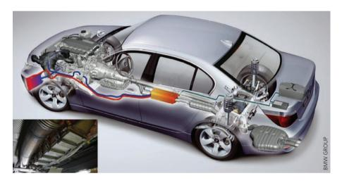
Figure 1 Integrating thermoelectrics into vehicles for improved fuel efficiency. Shown is a BMW 530i concept car with a thermoelectric generator (yellow; and inset) and radiator (red/blue).
